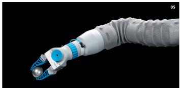
The interface between the tablet and the Festo Motion Terminal is the ROS (Robot Operating System) open source platform, on which the kinematics' path planning is calculated. In addition, the ROS interprets the incoming code from the tablet and forwards the resulting axis coordinates to the Motion Terminal.
