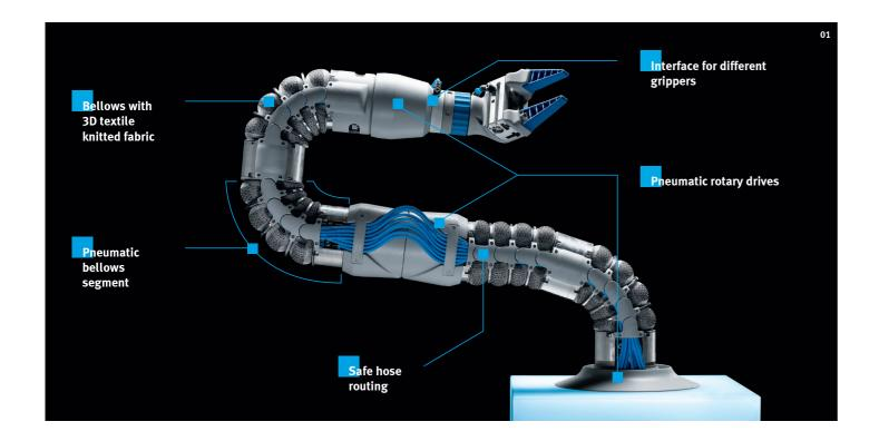
The pneumatic segments of the BionicSoftArm each have two bellows and a degree of freedom to keep the closed-loop control technology as simple as possible. However, by combining several bellows segments and rotary drives, its range of motion can be extended almost arbitrarily.
