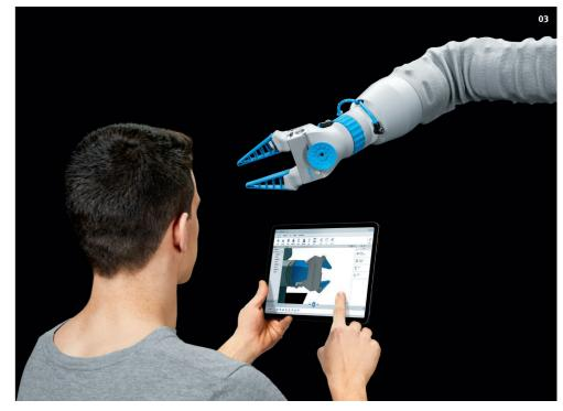
One robot arm, many variation possibilities: the BionicSoftArm is a compact further development of the BionicMotionRobot, whose range of applications has now been significantly expanded. This is made possible by the modular design of the BionicSoftArm, which can be combined from several pneumatic bellows segments and rotary drives. This enables it to master both free and flexible movements as well as defined sequences. At the same time, it is completely compliant and can work safely with people.
